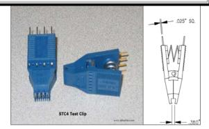
**STC4 IME Test Clip**: The STC4 IME Test Clip is designed for easy make and break electrical connections to unpackaged IME chips. The spring loaded clip open and close action assures a positive connect to all chip leads and provides for hands free testing of IMES.
