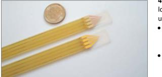
**4C Chip Carrier**: The 4C Chip Carrier is an 11.4 cm (4.5") long printed circuit board wand outfitted with pins at the upper end and bonding pads at the lower end.
