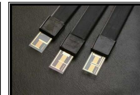
**INTERDIGITATED MICROSENSOR ELECTRODES (IMEs)**
