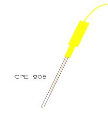
Electrode Body Total Length Lead Length Electrode Body O.D. Electrode Tip O.D. Immersion Depth Response Time Temperature Range pH Range Black Delrin 9.5 cm 1 m 2.5 mm 1.2 mm 2 mm 10 sec -4?C - 75?C 0 - 14
